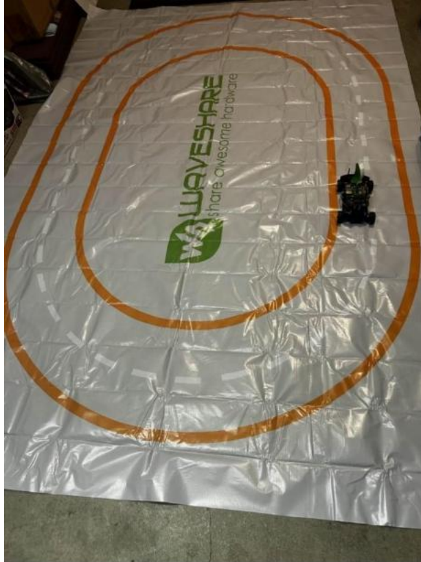
Figure 2: Testbed setup, Donkey Car placed on oval 3 by 2 meter track
