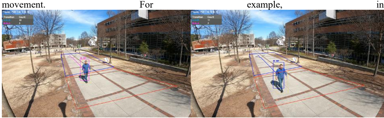
Figure 11 a person with Track ID 367 was initially in Zone A and later detected in Zone B, this would be logged as an A_to_B transition. Transition A_B: count increased from 10 to 11 from frame 708 to frame 709.
