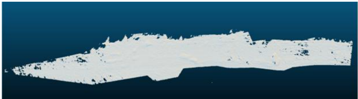
Figure 3: 3D point cloud road model, after cleaning and segmentation; Note the depressions in the center area of the model, which represent potholes in the road
