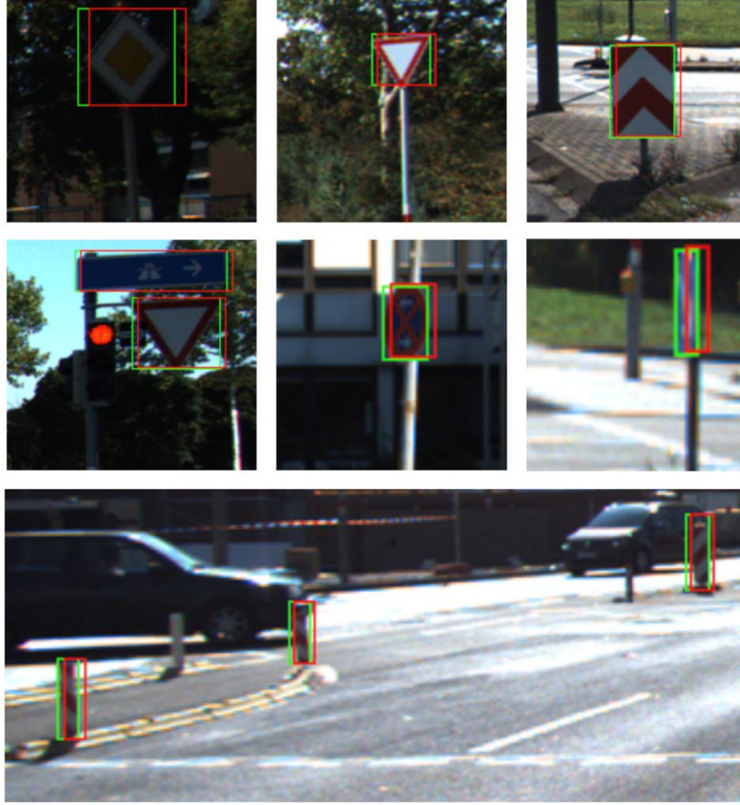
Figure 3 The original reprojection in red and the model output in green
