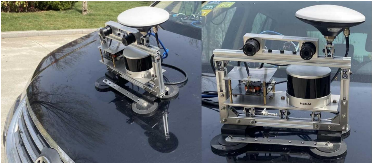
Figure C: Sensor Configuration from (RSXD, n.d.), composed of a LI-AR023ZWDR camera, Hesai XT32 LiDAR sensor, UBlox F9P GNSS-RTK, XSENS MTi670 IMU, and an ADXL345 Accelerometer
